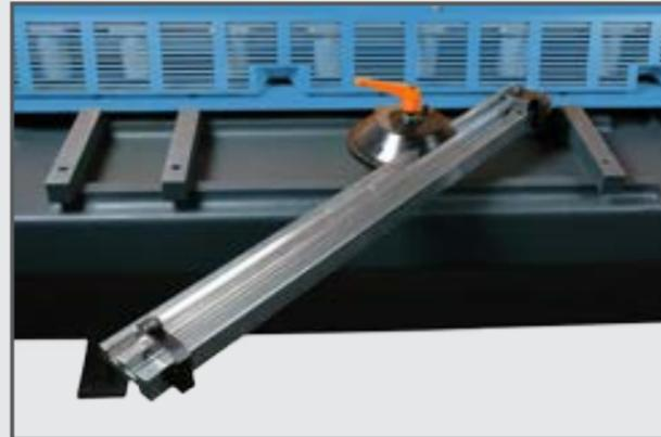
Protractor for Angle Shearing.
