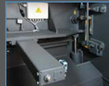
Motorised positioning with the SP9 preselection control or programmable positioning with the SC100 T control. Digital readout of the actual and pre-selected or programmed position. On the 6 mm models, motorised driven back gauge with a standard stroke of 750 mm and optional extension to 1000 mm. On the 12 mm model, motorised driven back gauge with standard stroke of 1000 mm.
